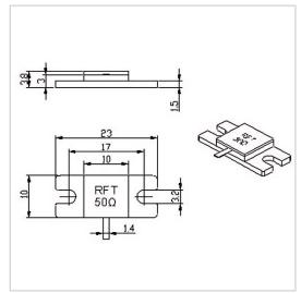
RF Solution offer a wide selection of Flanged Termination for global customers. RFT50-250TM2310 is a Flanged Termination in Frequency Range of DC $\sim$ 3.0 GHz. It is made of high quality materials under a high standard, the Resistance Range of this product is 50  $\Omega$ , Resistance Tolerance is  $\pm 5\%$  and VSWR Max is 1.20. The component has a good working performance and stability, it is ideal for handling a Power of 250 W.
