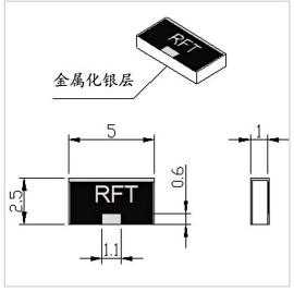
RF Solution offer a wide selection of Chip Termination for global customers. RFT50-20WT5025 is a Chip Termination in Frequency Range of DC $\sim$ 18.0 GHz. It is made of high quality materials under a high standard, the Resistance Range of this product is 50  $\Omega$ , Resistance Tolerance is  $\pm 5\%$  and VSWR Max is 1.20. The component has a good working performance and stability, it is ideal for handling a Power of 20 W.
