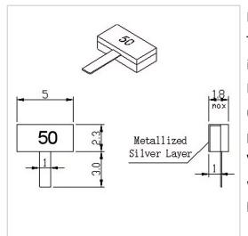
RF Solution offer a wide selection of Leaded Termination for global customers. RFT50-20TM5023 is a Leaded Termination in Frequency Range of DC~18.0 GHz. It is made of high quality materials under a high standard, the Resistance Range of this product is 50  $\Omega$ , Resistance Tolerance is ±5% and VSWR Max is 1.20~1.25. The component has a good working performance and stability, it is ideal for handling a Power of 20 W.
