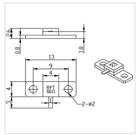
RF Solution offer a wide selection of Flanged Termination for global customers. RFT50-20TM1304 is a Flanged Termination in Frequency Range of DC $\sim$ 8.0 GHz. It is made of high quality materials under a high standard, the Resistance Range of this product is 50  $\Omega$ , Resistance Tolerance is  $\pm 5\%$  and VSWR Max is 1.20. The component has a good working performance and stability, it is ideal for handling a Power of 20 W.
