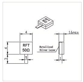
RF Solution offer a wide selection of Leaded Termination for global customers. RFT50-20TM0404 is a Leaded Termination in Frequency Range of DC~8.0 GHz. It is made of high quality materials under a high standard, the Resistance Range of this product is 50  $\Omega$ , Resistance Tolerance is  $\pm 5\%$  and VSWR Max is 1.20~1.25. The component has a good working performance and stability, it is ideal for handling a Power of 20 W.
