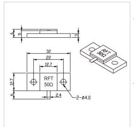
RF Solution offer a wide selection of Flanged Termination for global customers. RFT50-200TM3213B is a Flanged Termination in Frequency Range of DC~10.0 GHz. It is made of high quality materials under a high standard, the Resistance Range of this product is 50  $\Omega$ , Resistance Tolerance is ±5% and VSWR Max is 1.20~1.30. The component has a good working performance and stability, it is ideal for handling a Power of 200 W.
