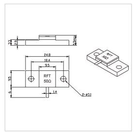
RF Solution offer a wide selection of Flanged Termination for global customers. RFT50-200TM2595 is a Flanged Termination in Frequency Range of DC $\sim$ 3.0 GHz. It is made of high quality materials under a high standard, the Resistance Range of this product is 50  $\Omega$ , Resistance Tolerance is  $\pm 5\%$  and VSWR Max is 1.20. The component has a good working performance and stability, it is ideal for handling a Power of 200 W.
