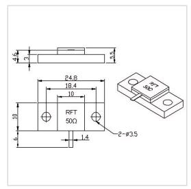
RF Solution offer a wide selection of Flanged Termination for global customers. RFT50-200TM2510 is a Flanged Termination in Frequency Range of DC $\sim$ 3.0 GHz. It is made of high quality materials under a high standard, the Resistance Range of this product is 50  $\Omega$ , Resistance Tolerance is  $\pm 5\%$  and VSWR Max is 1.20. The component has a good working performance and stability, it is ideal for handling a Power of 200 W.
