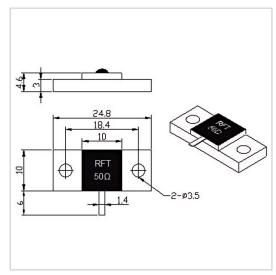
RF Solution offer a wide selection of Flanged Termination for global customers. RFT50-200TJ2510 is a Flanged Termination in Frequency Range of DC~4.0 GHz. It is made of high quality materials under a high standard, the Resistance Range of this product is 50  $\Omega$ , Resistance Tolerance is  $\pm 5\%$  and VSWR Max is 1.25. The component has a good working performance and stability, it is ideal for handling a Power of 200 W.
