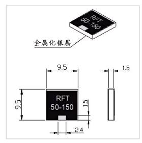
RF Solution offer a wide selection of Chip Termination for global customers. RFT50-150WT9595 is a Chip Termination in Frequency Range of DC $\sim$ 3.0 GHz. It is made of high quality materials under a high standard, the Resistance Range of this product is 50  $\Omega$ , Resistance Tolerance is  $\pm 5\%$  and VSWR Max is 1.20. The component has a good working performance and stability, it is ideal for handling a Power of 150 W.
