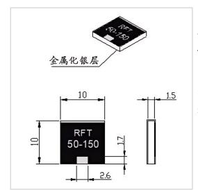
RF Solution offer a wide selection of Chip Termination for global customers. RFT50-150WT1010 is a Chip Termination in Frequency Range of DC~4.0 GHz. It is made of high quality materials under a high standard, the Resistance Range of this product is 50  $\Omega$ , Resistance Tolerance is ±5% and VSWR Max is 1.25. The component has a good working performance and stability, it is ideal for handling a Power of 150 W.
