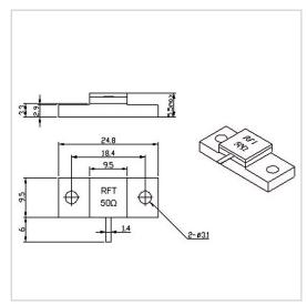
RF Solution offer a wide selection of Flanged Termination for global customers. RFT50-150TM2595 is a Flanged Termination in Frequency Range of DC $\sim$ 3.0 GHz. It is made of high quality materials under a high standard, the Resistance Range of this product is 50  $\Omega$ , Resistance Tolerance is  $\pm 5\%$  and VSWR Max is 1.20. The component has a good working performance and stability, it is ideal for handling a Power of 150 W.
