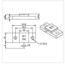
RF Solution offer a wide selection of Flanged Termination for global customers. RFT50-150TM2510 is a Flanged Termination in Frequency Range of DC $\sim$ 3.0 GHz. It is made of high quality materials under a high standard, the Resistance Range of this product is 50  $\Omega$ , Resistance Tolerance is  $\pm 5\%$  and VSWR Max is 1.20. The component has a good working performance and stability, it is ideal for handling a Power of 150 W.
