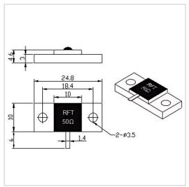
RF Solution offer a wide selection of Flanged Termination for global customers. RFT50-150TJ2510 is a Flanged Termination in Frequency Range of DC~4.0 GHz. It is made of high quality materials under a high standard, the Resistance Range of this product is 50  $\Omega$ , Resistance Tolerance is  $\pm 5\%$  and VSWR Max is 1.25. The component has a good working performance and stability, it is ideal for handling a Power of 150 W.
