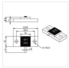
RF Solution offer a wide selection of Flanged Termination for global customers. RFT50-150TJ2510B is a Flanged Termination in Frequency Range of DC~7.0 GHz. It is made of high quality materials under a high standard, the Resistance Range of this product is 50  $\Omega$ , Resistance Tolerance is  $\pm 5\%$  and VSWR Max is 1.20~1.30. The component has a good working performance and stability, it is ideal for handling a Power of 150 W.
