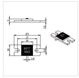
RF Solution offer a wide selection of Flanged Termination for global customers. RFT50-150TJ2310B is a Flanged Termination in Frequency Range of DC~7.0 GHz. It is made of high quality materials under a high standard, the Resistance Range of this product is 50  $\Omega$ , Resistance Tolerance is  $\pm 5\%$  and VSWR Max is 1.20~1.30. The component has a good working performance and stability, it is ideal for handling a Power of 150 W.
