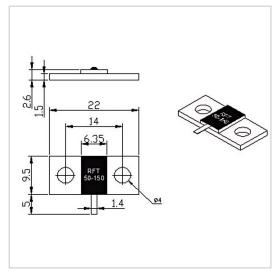
RF Solution offer a wide selection of Flanged Termination for global customers. RFT50-150TJ2295 is a Flanged Termination in Frequency Range of DC $\sim$ 3.0 GHz. It is made of high quality materials under a high standard, the Resistance Range of this product is 50  $\Omega$ , Resistance Tolerance is  $\pm 5\%$  and VSWR Max is 1.25. The component has a good working performance and stability, it is ideal for handling a Power of 150 W.
