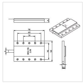
RF Solution offer a wide selection of Flanged Termination for global customers. RFT50-1500TM5078 is a Flanged Termination in Frequency Range of DC~800 MHz. It is made of high quality materials under a high standard, the Resistance Range of this product is 50  $\Omega$ , Resistance Tolerance is  $\pm 5\%$  and VSWR Max is 1.30. The component has a good working performance and stability, it is ideal for handling a Power of 1500 W.
