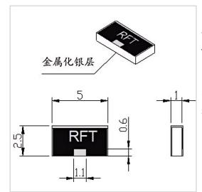
RF Solution offer a wide selection of Chip Termination for global customers. RFT50-10WT5025 is a Chip Termination in Frequency Range of DC~18.0 GHz. It is made of high quality materials under a high standard, the Resistance Range of this product is 50  $\Omega$ , Resistance Tolerance is ±5% and VSWR Max is 1.20~1.25. The component has a good working performance and stability, it is ideal for handling a Power of 10 W.
