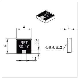
RF Solution offer a wide selection of Chip Termination for global customers. RFT50-10WT0404 is a Chip Termination in Frequency Range of DC $\sim$ 8.0 GHz. It is made of high quality materials under a high standard, the Resistance Range of this product is 50  $\Omega$ , Resistance Tolerance is  $\pm 5\%$  and VSWR Max is  $1.20\sim1.25$ . The component has a good working performance and stability, it is ideal for handling a Power of 10 W.
