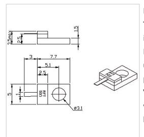
RF Solution offer a wide selection of Flanged Termination for global customers. RFT50-10TM7750I is a Flanged Termination in Frequency Range of DC~18.0 GHz. It is made of high quality materials under a high standard, the Resistance Range of this product is 50  $\Omega$ , Resistance Tolerance is ±5% and VSWR Max is 1.20~1.30. The component has a good working performance and stability, it is ideal for handling a Power of 10 W.
