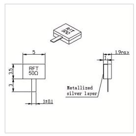
RF Solution offer a wide selection of Leaded Termination for global customers. RFT50-10TM5035 is a Leaded Termination in Frequency Range of DC~10.0 GHz. It is made of high quality materials under a high standard, the Resistance Range of this product is 50  $\Omega$ , Resistance Tolerance is  $\pm 5\%$  and VSWR Max is 1.20~1.25. The component has a good working performance and stability, it is ideal for handling a Power of 10 W.
