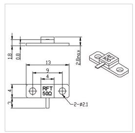
RF Solution offer a wide selection of Flanged Termination for global customers. RFT50-10TM1304 is a Flanged Termination in Frequency Range of DC $\sim$ 8.0 GHz. It is made of high quality materials under a high standard, the Resistance Range of this product is 50  $\Omega$ , Resistance Tolerance is  $\pm 5\%$  and VSWR Max is 1.20. The component has a good working performance and stability, it is ideal for handling a Power of 10 W.
