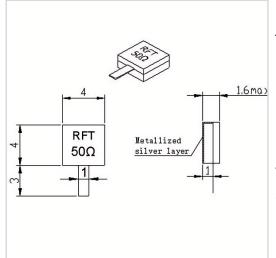
RF Solution offer a wide selection of Leaded Termination for global customers. RFT50-10TM0404 is a Leaded Termination in Frequency Range of DC~8.0 GHz. It is made of high quality materials under a high standard, the Resistance Range of this product is 50  $\Omega$ , Resistance Tolerance is ±5% and VSWR Max is 1.20. The component has a good working performance and stability, it is ideal for handling a Power of 10 W.
