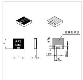
RF Solution offer a wide selection of Chip Termination for global customers. RFT50-10CT0404 is a Chip Termination in Frequency Range of DC $\sim$ 10.0 GHz. It is made of high quality materials under a high standard, the Resistance Range of this product is 50  $\Omega$ , Resistance Tolerance is  $\pm 5\%$  and VSWR Max is  $1.20\sim1.30$ . The component has a good working performance and stability, it is ideal for handling a Power of 10 W.
