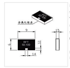
RF Solution offer a wide selection of Chip Termination for global customers. RFT50-100WT0906C is a Chip Termination in Frequency Range of DC~8.0 GHz. It is made of high quality materials under a high standard, the Resistance Range of this product is 50  $\Omega$ , Resistance Tolerance is ±5% and VSWR Max is 1.25. The component has a good working performance and stability, it is ideal for handling a Power of 100 W.
