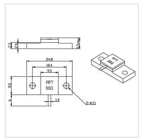
RF Solution offer a wide selection of Flanged Termination for global customers. RFT50-100TM2595 is a Flanged Termination in Frequency Range of DC $\sim$ 3.0 GHz. It is made of high quality materials under a high standard, the Resistance Range of this product is 50  $\Omega$ , Resistance Tolerance is  $\pm 5\%$  and VSWR Max is 1.20. The component has a good working performance and stability, it is ideal for handling a Power of 100 W.
