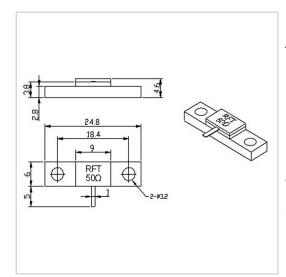
RF Solution offer a wide selection of Flanged Termination for global customers. RFT50-100TM2506 is a Flanged Termination in Frequency Range of DC~4.0 GHz. It is made of high quality materials under a high standard, the Resistance Range of this product is 50  $\Omega$ , Resistance Tolerance is ±5% and VSWR Max is 1.20. The component has a good working performance and stability, it is ideal for handling a Power of 100 W.
