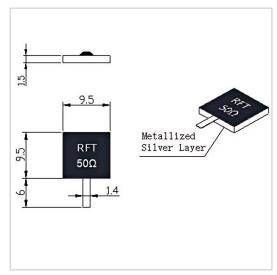
RF Solution offer a wide selection of Leaded Termination for global customers. RFT50-100TJ9595 is a Leaded Termination in Frequency Range of DC $\sim$ 3.0 GHz. It is made of high quality materials under a high standard, the Resistance Range of this product is 50  $\Omega$ , Resistance Tolerance is  $\pm 5\%$  and VSWR Max is 1.20. The component has a good working performance and stability, it is ideal for handling a Power of 100 W.
