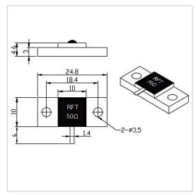
RF Solution offer a wide selection of Flanged Termination for global customers. RFT50-100TJ2510 is a Flanged Termination in Frequency Range of DC~4.0 GHz. It is made of high quality materials under a high standard, the Resistance Range of this product is 50  $\Omega$ , Resistance Tolerance is  $\pm 5\%$  and VSWR Max is 1.25. The component has a good working performance and stability, it is ideal for handling a Power of 100 W.
