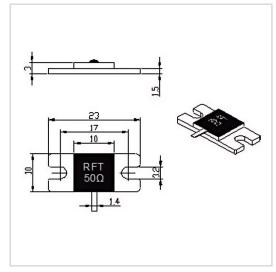
RF Solution offer a wide selection of Flanged Termination for global customers. RFT50-100TJ2310 is a Flanged Termination in Frequency Range of DC~4.0 GHz. It is made of high quality materials under a high standard, the Resistance Range of this product is 50  $\Omega$ , Resistance Tolerance is  $\pm 5\%$  and VSWR Max is 1.20. The component has a good working performance and stability, it is ideal for handling a Power of 100 W.
