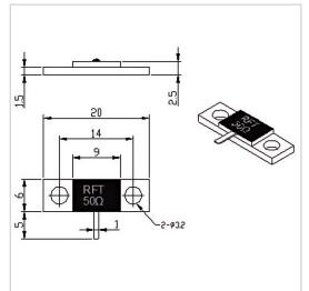
RF Solution offer a wide selection of Flanged Termination for global customers. RFT50-100TJ2006 is a Flanged Termination in Frequency Range of DC~4.0 GHz. It is made of high quality materials under a high standard, the Resistance Range of this product is 50  $\Omega$ , Resistance Tolerance is ±5% and VSWR Max is 1.20. The component has a good working performance and stability, it is ideal for handling a Power of 100 W.
