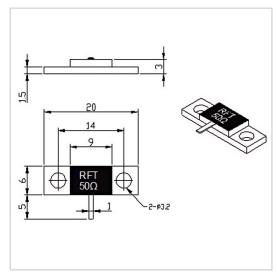
RF Solution offer a wide selection of Flanged Termination for global customers. RFT50-100TJ2006C is a Flanged Termination in Frequency Range of DC~8.0 GHz. It is made of high quality materials under a high standard, the Resistance Range of this product is 50  $\Omega$ , Resistance Tolerance is  $\pm 5\%$  and VSWR Max is 1.25. The component has a good working performance and stability, it is ideal for handling a Power of 100 W.
