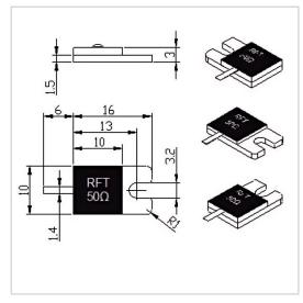
RF Solution offer a wide selection of Flanged Termination for global customers. RFT50-100TJ1610 is a Flanged Termination in Frequency Range of DC~4.0 GHz. It is made of high quality materials under a high standard, the Resistance Range of this product is 50  $\Omega$ , Resistance Tolerance is  $\pm 5\%$  and VSWR Max is 1.25. The component has a good working performance and stability, it is ideal for handling a Power of 100 W.
