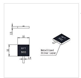
RF Solution offer a wide selection of Leaded Termination for global customers. RFT50-100TJ1010 is a Leaded Termination in Frequency Range of DC~3.0 GHz. It is made of high quality materials under a high standard, the Resistance Range of this product is 50  $\Omega$ , Resistance Tolerance is ±5% and VSWR Max is 1.20. The component has a good working performance and stability, it is ideal for handling a Power of 100 W.
