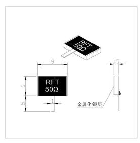
RF Solution offer a wide selection of Leaded Termination for global customers. RFT50-100TJ0906C is a Leaded Termination in Frequency Range of DC~8.0 GHz. It is made of high quality materials under a high standard, the Resistance Range of this product is 50  $\Omega$ , Resistance Tolerance is  $\pm 5\%$  and VSWR Max is 1.25. The component has a good working performance and stability, it is ideal for handling a Power of 100 W.
