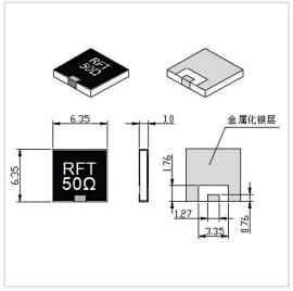
RF Solution offer a wide selection of Chip Termination for global customers. RFT50-100CT6363 is a Chip Termination in Frequency Range of DC $\sim$ 6.0 GHz. It is made of high quality materials under a high standard, the Resistance Range of this product is 50  $\Omega$ , Resistance Tolerance is  $\pm 5\%$  and VSWR Max is  $1.20\sim1.25$ . The component has a good working performance and stability, it is ideal for handling a Power of 100 W.
