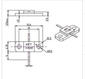
RF Solution offer a wide selection of Flanged Attenuator for global customers. RFT20N-60AM1663-6 is a Flanged Attenuator in Frequency Range of DC~6.0 GHz. It is made of high quality materials under a high standard, the Attenuation Value of this product is 20 dB, Attenuation Tolerance is  $\pm 0.8$  dB and VSWR Max is 1.25. The component has a good working performance and stability, it is ideal for handling a Rated Power of 60 W.
