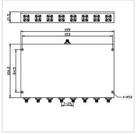
RF Solution offer a wide selection of 8 Ways Power Divider for global customers. PD08-F2011-N-690-2700MHz is a 8 Ways Power Divider in Frequency Range of 690~2700 MHz. It is made of high quality materials under a high standard, the Insertion Loss Max of this product is 1.1 dB, Isolation Min is 18 dB and Split Loss is 9.0 dB. The component has a good working performance and stability, it is ideal for handling a Rated Power of 50 W.
