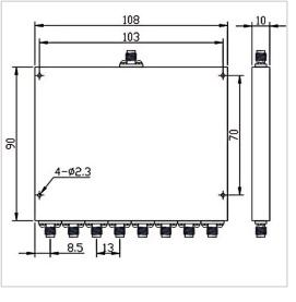
RF Solution offer a wide selection of 8 Ways Power Divider for global customers. PD08-F1190-S-500-4000MHz is a 8 Ways Power Divider in Frequency Range of 500~4000 MHz. It is made of high quality materials under a high standard, the Insertion Loss Max of this product is 1.8 dB (Excluding 3.0dB separation loss), Isolation Min is 18 dB and Amplitude Unbalance is ±0.5 dB. The component has a good working performance and stability, it is ideal for handling a Forward Power of 20 W.
