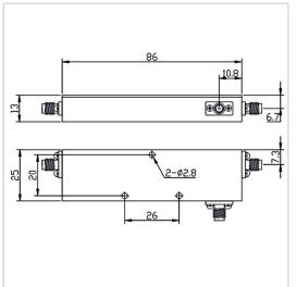
RF Solution offer a wide selection of Coupler for global customers. PD06-F2586-S-0.698-2.2GHz is a Coupler in Frequency Range of 0.698~2.2 GHz. It is made of high quality materials under a high standard, the Insertion Loss Max of this product is 0.4 dB , Nominal Coupling is  $6\pm 1$  dB and Coupling Sensitivity Max is  $\pm 0.3$  dB. The component has a good working performance and stability, it is ideal for handling a Rated Power of 50 W.
