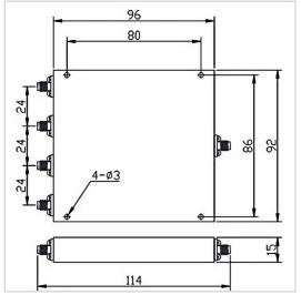
RF Solution offer a wide selection of 4 Ways Power Divider for global customers. PD04-F9296-S-698-3800MHz is a 4 Ways Power Divider in Frequency Range of 698~3800 MHz. It is made of high quality materials under a high standard, the Insertion Loss Max of this product is 1.2 dB, Isolation Min is 20 dB and Split Loss is 6.0 dB. The component has a good working performance and stability, it is ideal for handling a Rated Power of 50 W.
