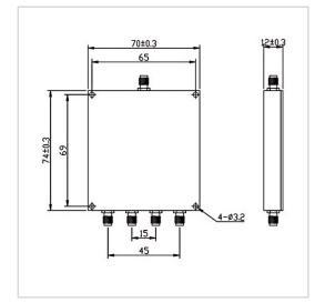
RF Solution offer a wide selection of 4 Ways Power Divider for global customers. PD04-F7074-S-500-2500MHz is a 4 Ways Power Divider in Frequency Range of 500~2500 MHz. It is made of high quality materials under a high standard, the Insertion Loss Max of this product is 1.2 dB, Isolation Min is 20 dB and Split Loss is 6.0 dB. The component has a good working performance and stability, it is ideal for handling a Forward Power of 40 W.
