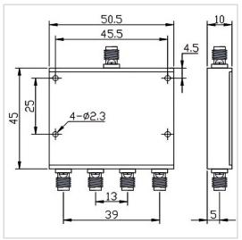
RF Solution offer a wide selection of 4 Ways Power Divider for global customers. PD04-F5045-S-6-18GHz is a 4 Ways Power Divider in Frequency Range of  $6.0{\sim}18.0$  GHz. It is made of high quality materials under a high standard, the Insertion Loss Max of this product is 1.2 dB, Isolation Min is 18 dB and Amplitude Unbalance is  $\pm 0.5$  dB. The component has a good working performance and stability, it is ideal for handling a Forward Power of 20 W.
