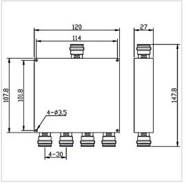
RF Solution offer a wide selection of 4 Ways Power Divider for global customers. PD04-F1211-M-698-4000MHz is a 4 Ways Power Divider in Frequency Range of 698~4000 MHz. It is made of high quality materials under a high standard, the Insertion Loss Max of this product is 1.2 dB, Isolation Min is 20 dB and Split Loss is 6.0 dB. The component has a good working performance and stability, it is ideal for handling a Rated Power of 1 W.
