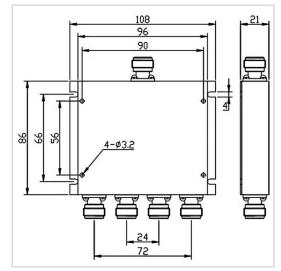
RF Solution offer a wide selection of 4 Ways Power Divider for global customers. PD04-F1186-N-698-3800MHz is a 4 Ways Power Divider in Frequency Range of 698~3800 MHz. It is made of high quality materials under a high standard, the Insertion Loss Max of this product is 1.2 dB, Isolation Min is 20 dB and Split Loss is 6.0 dB. The component has a good working performance and stability, it is ideal for handling a Rated Power of 50 W.
