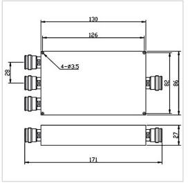
RF Solution offer a wide selection of 3 Ways Power Divider for global customers. PD03-F8613-N-698-3800MHz is a 3 Ways Power Divider in Frequency Range of 698~3800 MHz. It is made of high quality materials under a high standard, the Insertion Loss Max of this product is 1.2 dB, Isolation Min is 20 dB and Split Loss is 4.8 dB. The component has a good working performance and stability, it is ideal for handling a Rated Power of 50 W.
