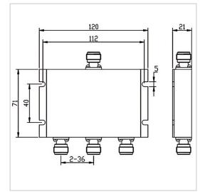
RF Solution offer a wide selection of 3 Ways Power Divider for global customers. PD03-F1271-N-136-174MHz is a 3 Ways Power Divider in Frequency Range of 176~174 MHz. It is made of high quality materials under a high standard, the Insertion Loss Max of this product is 0.4 dB, Isolation Min is 20 dB and Split Loss is 4.8 dB. The component has a good working performance and stability, it is ideal for handling a Rated Power of 50 W.
