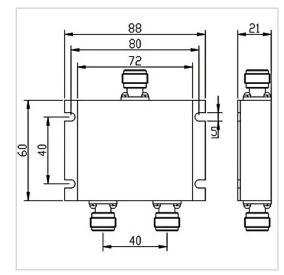
RF Solution offer a wide selection of 2 Ways Power Divider for global customers. PD02-F8860-N-136-174MHz is a 2 Ways Power Divider in Frequency Range of 134~174 MHz. It is made of high quality materials under a high standard, the Split Loss of this product is 3.0 dB, Insertion Loss Max is 0.3 dB and Isolation Min is 18.0 dB. The component has a good working performance and stability, it is ideal for handling a Forward Power of 20 W.
