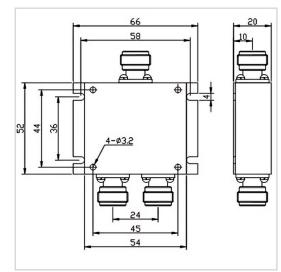
RF Solution offer a wide selection of 2 Ways Power Divider for global customers. PD02-F6652-N-698-3800MHz is a 2 Ways Power Divider in Frequency Range of 698~3800 MHz. It is made of high quality materials under a high standard, the Insertion Loss Max of this product is 0.8 dB, Split Loss is 3.5 dB and Isolation Min is 20 dB. The component has a good working performance and stability, it is ideal for handling a Rated Power of 50 W.
